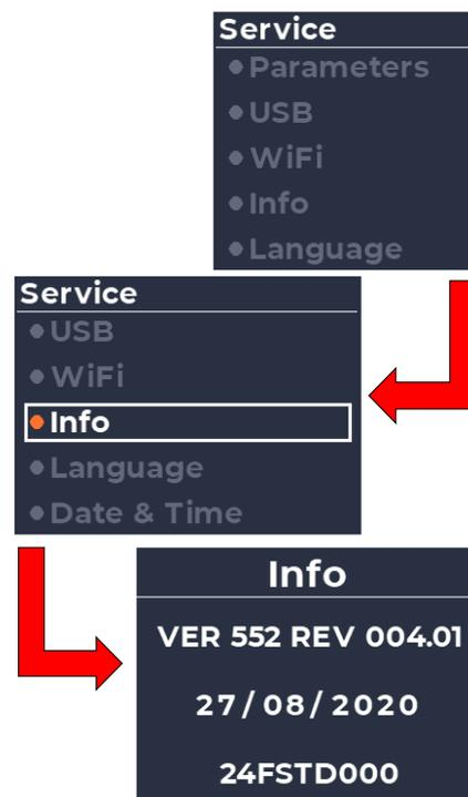
The diagram shows the navigation path for viewing the firmware version. It starts with a 'Service' menu containing 'Parameters', 'USB', 'WiFi', 'Info', and 'Language'. A red arrow points to the 'Info' option. The next screen shows 'Service' with 'USB', 'WiFi', 'Info' (highlighted), 'Language', and 'Date & Time'. A red arrow points to the 'Info' option. The final screen shows the 'Info' screen with the following text: 'VER 552 REV 004.01', '27/08/2020', and '24FSTD000'.
